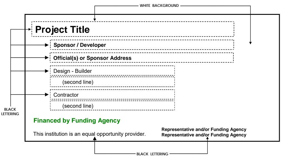
SIGN DIMENSIONS: 1200 mm x 2400 mm x 19 mm (approx. 4' x 8' x ¾") PLYWOOD PANEL (APA RATED A-B GRADE-EXTERIOR)
